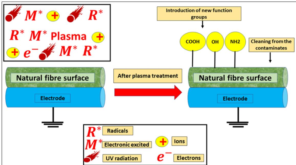
Figure 3: Schematic representation of the plasma surface treatment.
