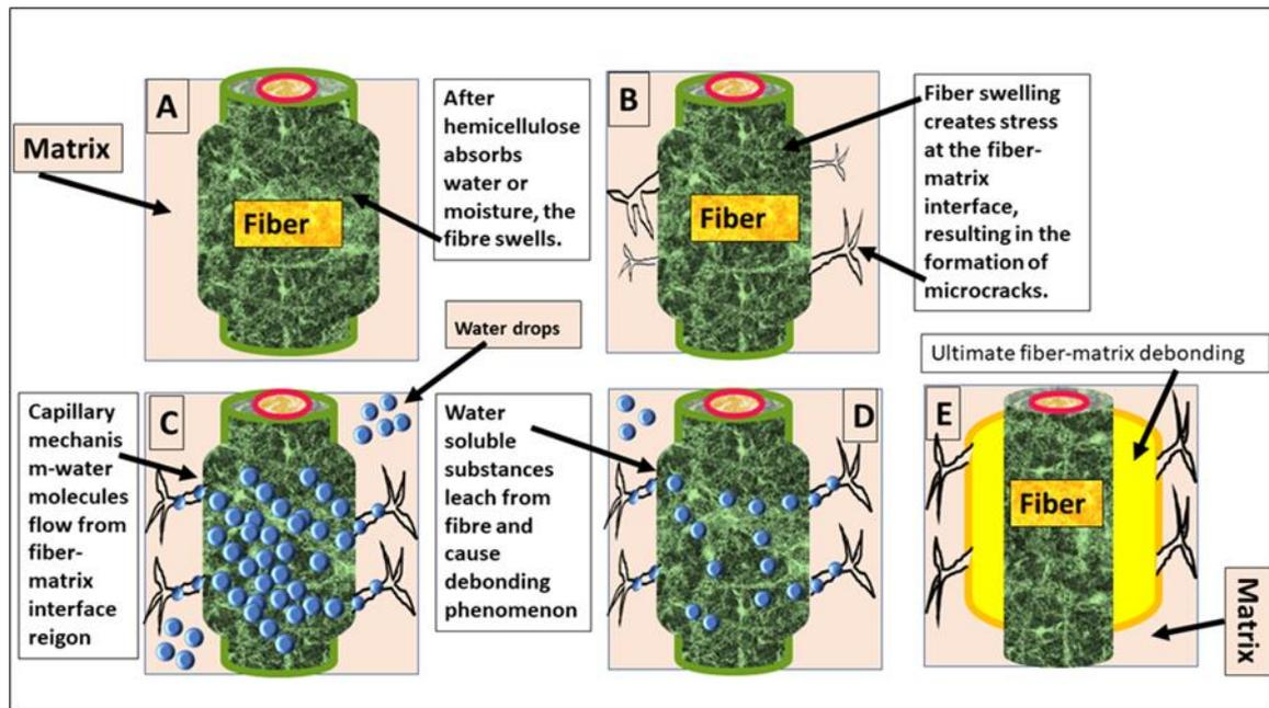
**Figure 1:** Schematic Representation of Effect of Water on Fiber-Matrix Interface.
