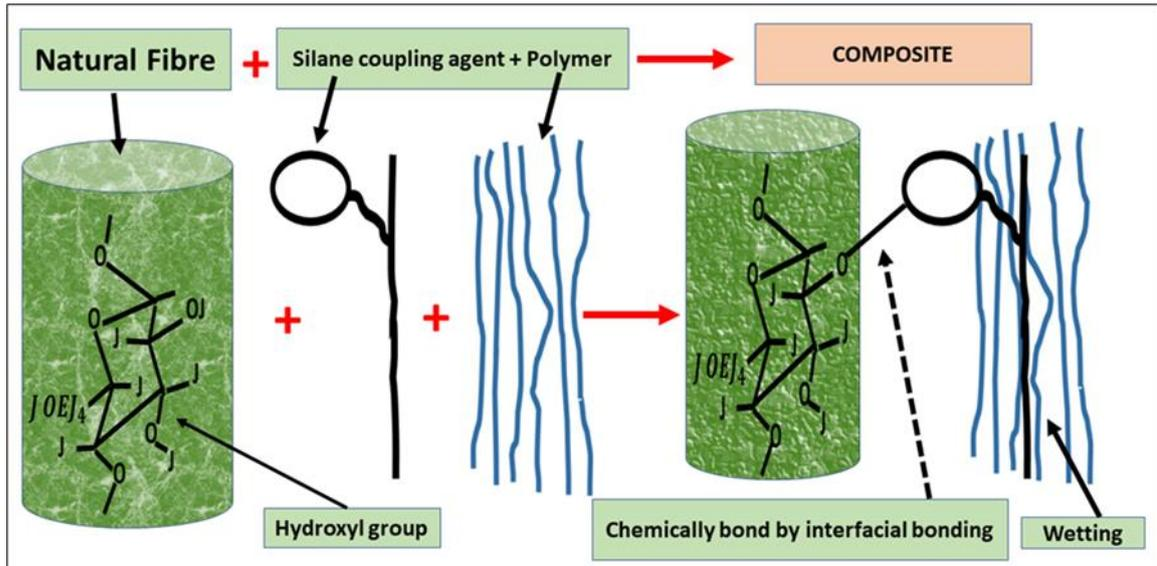
Figure 2: Schematic representation of silane treatment.
