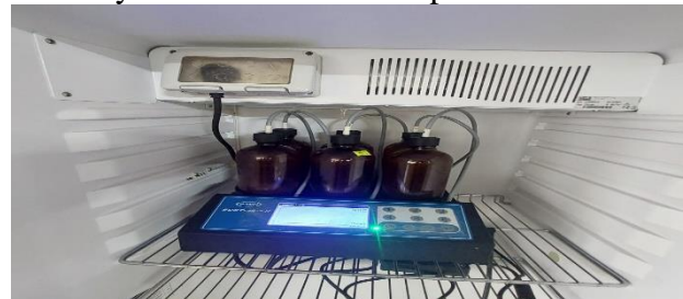
Figure 3 Biochemical Oxygen Demand (BOD) test.
