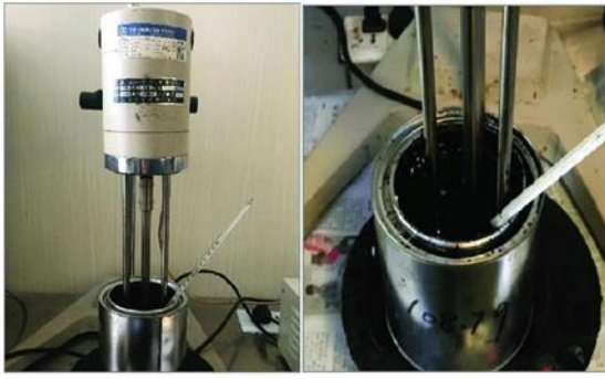
Figure 2: Preparation of modified HMA using high-speed shear mixer.
