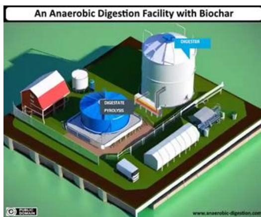
Fig.1 An anaerobic digestion plant with biochar addition from digestate pyrolysis. (source: reference [4]).
