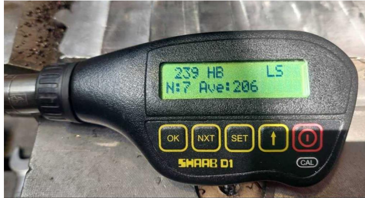
Figure 2. Brinell hardness testing procedure on the 316L stainless steel sample
