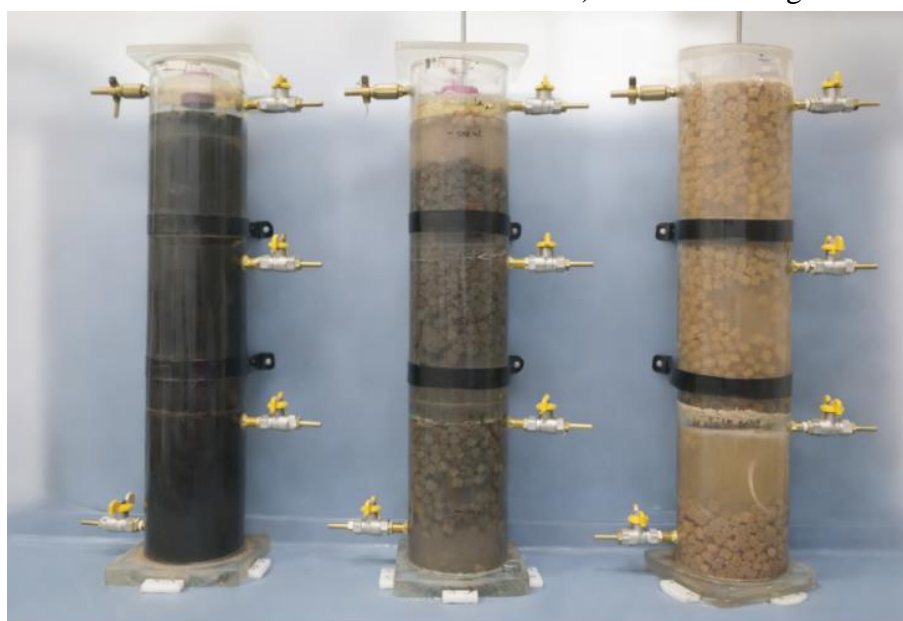
Figure 1: combined activated sludge-moving bed biofilm reactor(AS-MBBR )
