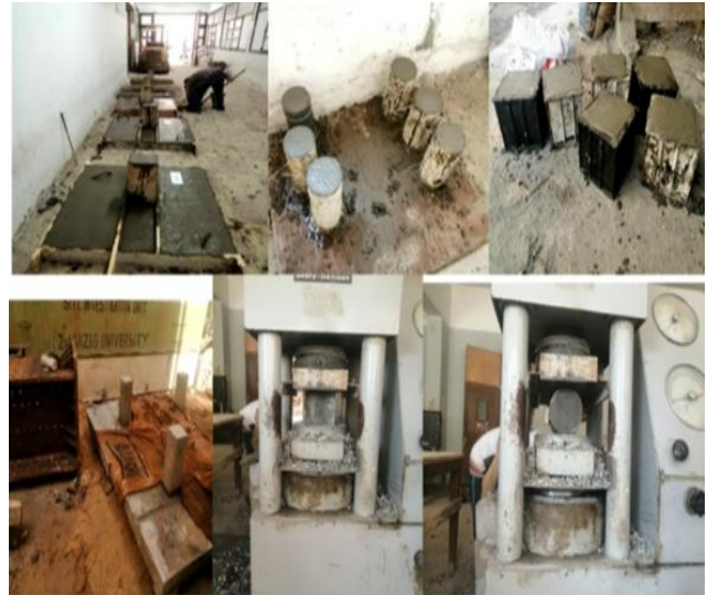
Figure 15. Casting curing, and testing of specimens [48]
