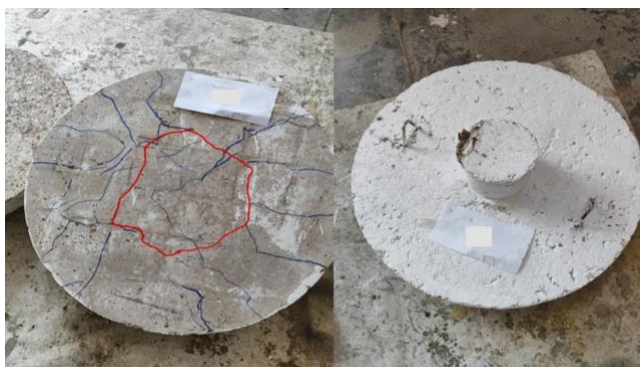
Figure 16. Crack pattern for circular specimen [49]
