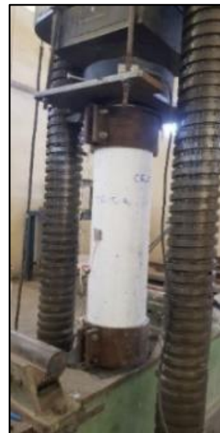
Figure 6. Tested Column Specimens Set Up
