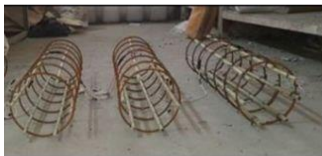
Figure 2. GFRP and Steel Bar Distribution
