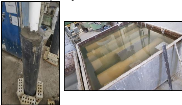
Figure 4. Column Specimens' Casting, Processing, and Curing
