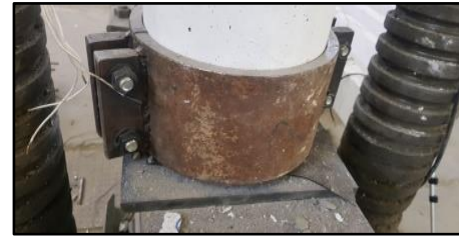
Figure 5. Specimens' Steel Caps
