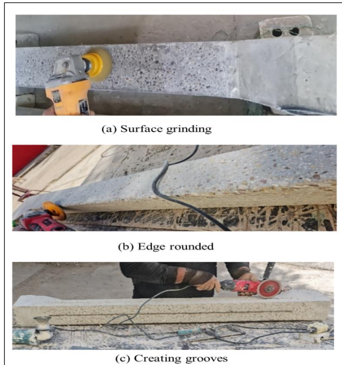
Figure 2. Process of strengthening modification
