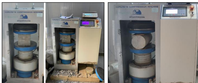
Figure 6. Compression Strength Test for Cube and Splitting Tensile Strength Test for Cylinder Samples
