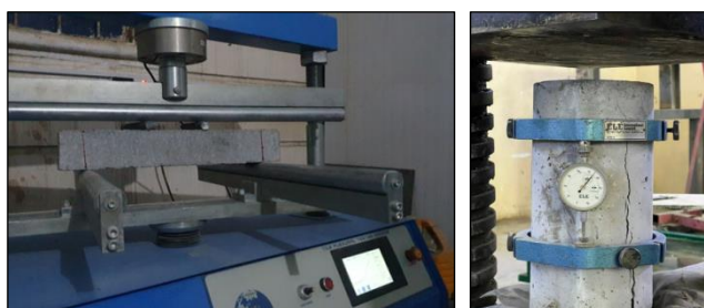
Figure 7. Flexural Strength Test for Prism and Test of the Modulus of Elasticity
