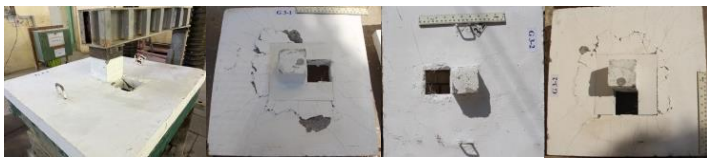
Figure 11. Compression and Tension Face for Slab G3-1,
