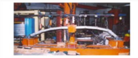
Figure 5. Structural Failure in Composite Arches
